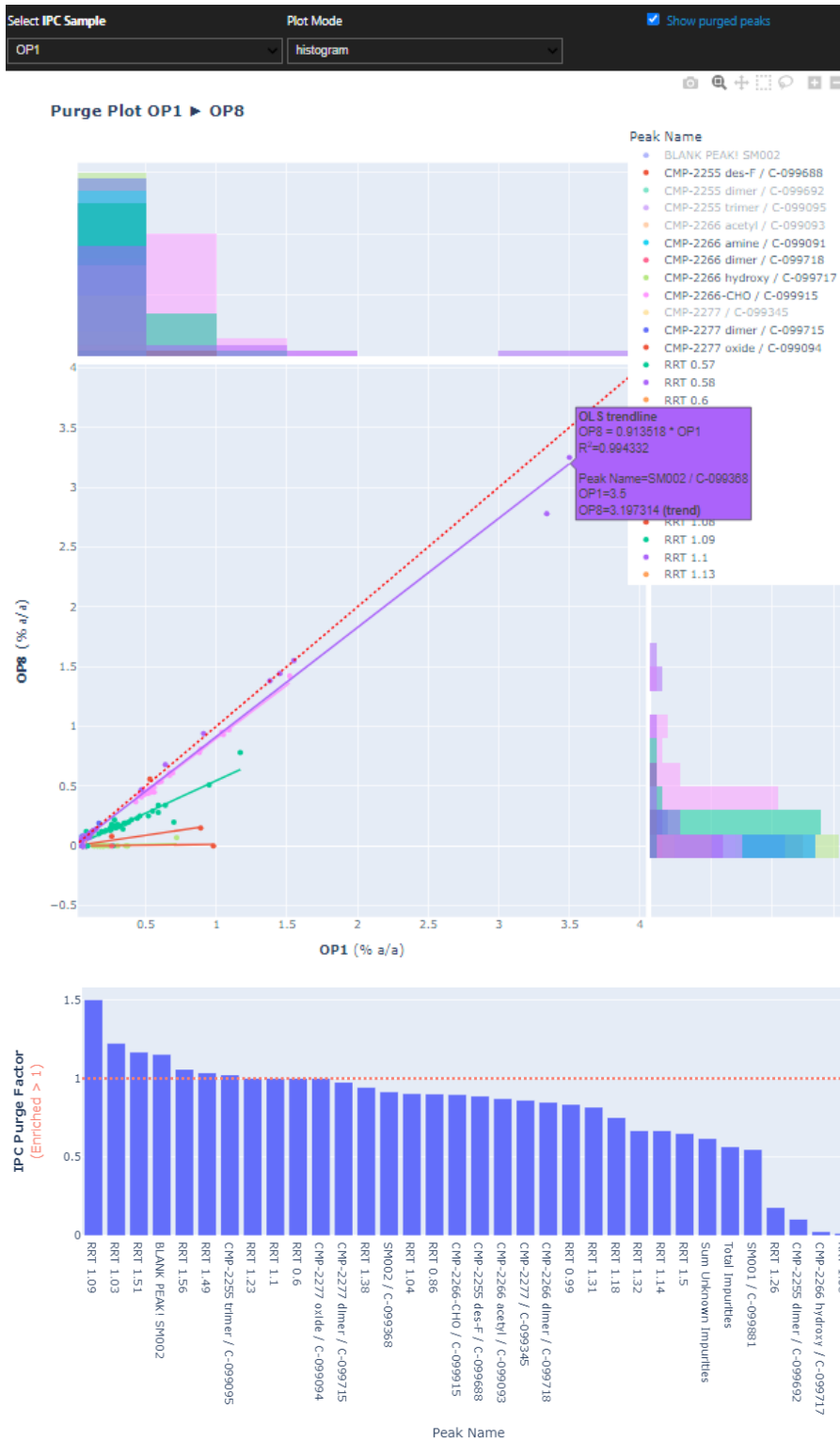
Figure 6: IPC Purge Factors between any two points in the process are obtained based on linear regression (top) and summarised in a bar plot (bottom). The example here shows purge factors across 8 extraction steps.
