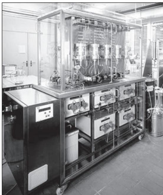
Figure 2 – Simulated Moving Bed (SMB) set-up
