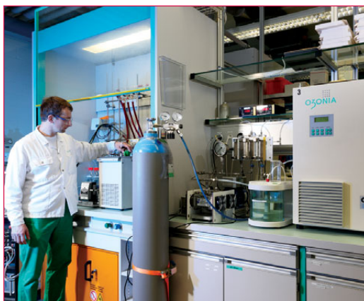
Carbogen Amcis carries out ozonolysis in flow at its early phase process R&D labs in Neuland
