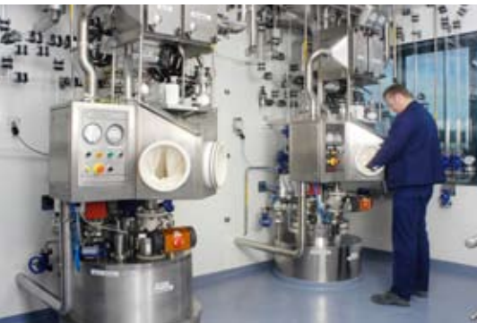
Picture 2: Reactors in CARBOGEN AMCIS' small-scale Bubendorf facility for highly potent APIs.
